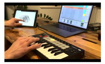
Figure 4: Setup using an iPad for sketch input that sends OSC messages to a Max4Live patch to manipulate synthesised sound in Ableton Live for a demonstration that can be viewed at https://youtu.be/4Yzv2rgTgOE.
